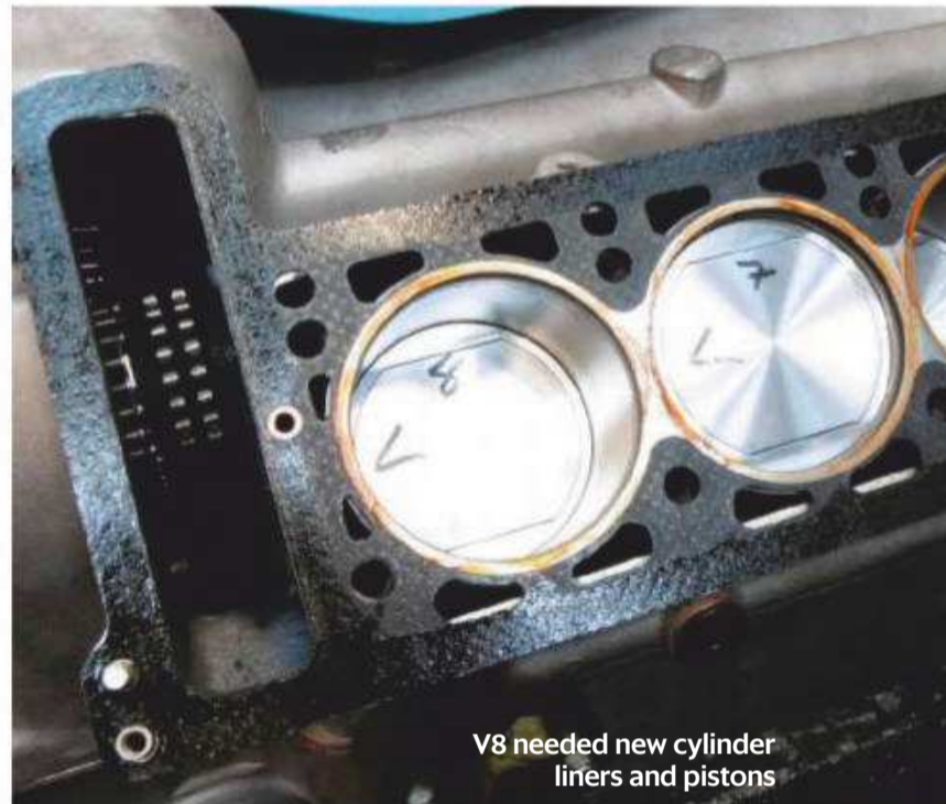
Alloy cylinder head and block were resin treated to resist porosity
