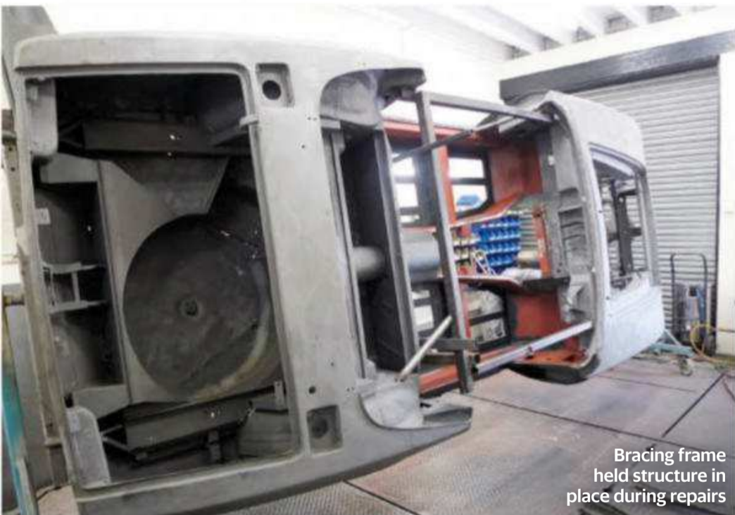
Most of the lower metalwork had to be remade
